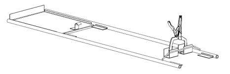
Insert the corrugation support of the platform into the panel corrugation at the eave and rotate the platform down onto the pan.
