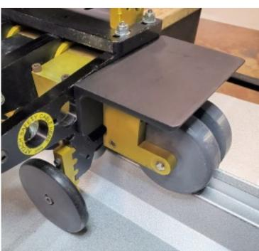
Apply downward pressure to the pressure plate as needed. This is typically at startup, end laps, and areas where there may be panel separation.
