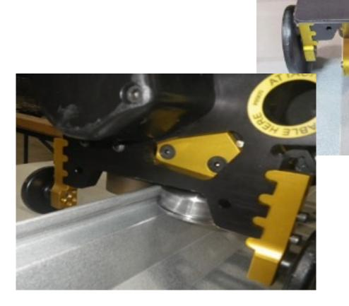
The pictures above detail how the seam should look when entering and exiting the machine. While seaming the female side guide wheel (indicated by the yellow arrow) should always be turning. If it stops turning, apply downward pressure to the pressure plate until it resumes. If this does not work, stop the machine and inspect the area for issues. Restart once the problem has been identified and corrected.
