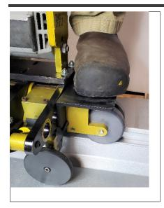
At all panel end laps, press down on the machine's pressure plate to help ensure it does not ride off the seam. This also needs to be done in any area where there is panel separation.
