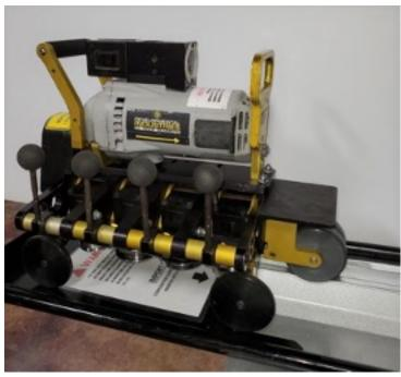
Again, **NEVER** straddle or stand on the platform and always wear proper fall protection. Be sure to attach a tether to the seamer any time it is on the roof to prevent it from falling off. Failure to do so could result in machine damage, serious injury, and/or death.
