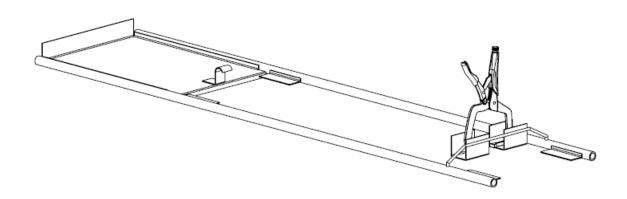
Before beginning the seaming process, crimp the ends of the panels together using the starter hand clamp. Then place the clamp on the horizontal legs flush with the starting end of the panel. With the starter tool, fold the seam over the clamp to a 90° position as shown below.
