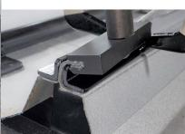
A seamer starting platform is available for purchase from D.I. Roof Seamers. This can be used to hold the machine in the correct starting position beyond the eave of the building. This platform should **NEVER**
