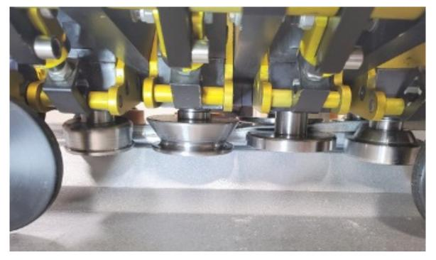
The seamer must be engaged in this manner. Failure to do so will result in panel damage.
