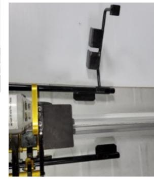
Run the seamer approximately 12" to ensure that you are receiving the desired seaming operation. If there are any issues, stop immediately and contact D.I. Technical Support at 1-888-343-0456.
